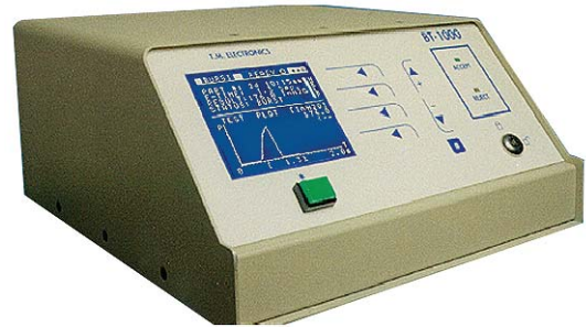
The TME BT-1000 performs both seal strength & package integrity testing
